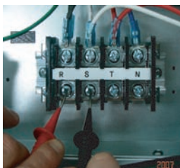
* Measuring input voltage
