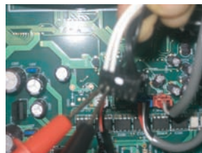
Check the resistance of constant compressor discharge temperature sensor
