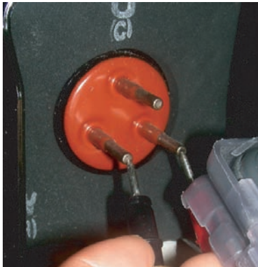
* Measuring resistance between each terminal of compressor
